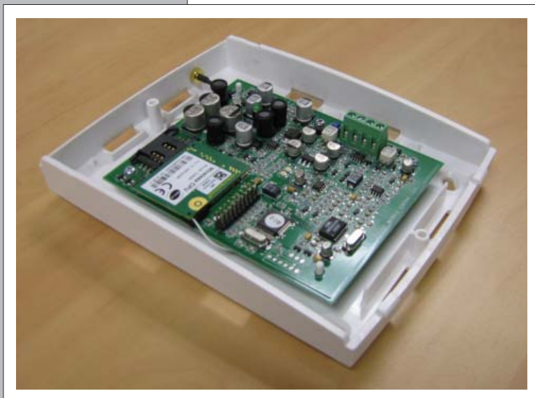
GSM Terminal Block
